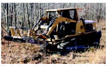
A brush-cutting machine is used to mow down brush and small trees. The cutter can mow down trees with up to a 4-inch diameter.
